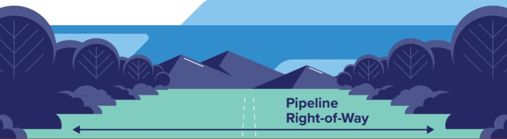
Pipelines are found in a space called the Right-of-Way (ROW). A pipeline ROW, or easement, is a strip of land above and around a gas pipeline. In this area, the property owner gives some legal rights to the pipeline operator so they can inspect and maintain the pipeline to ensure safe operation.
